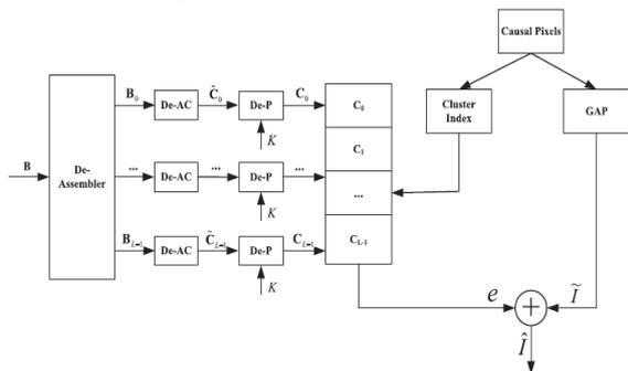
Fig. 5. Schematic diagram of sequential decryption and decompression.
