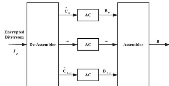
Fig. 4. Schematic diagram of compressing the encrypted data.
