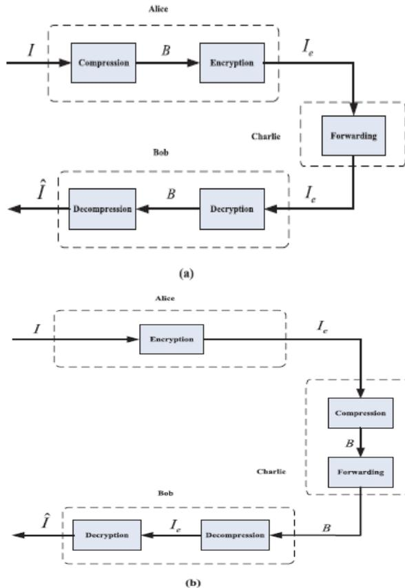
Fig. 1. (a) Traditional Compression-then-Encryption (CTE) system;
