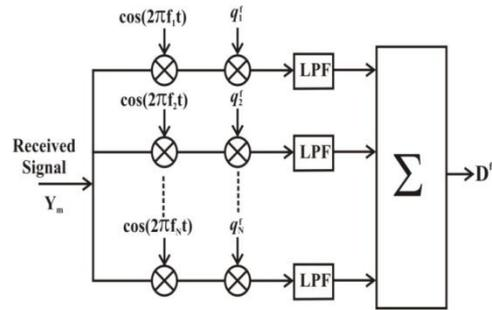
Fig.2.2 Receiver of MC-CDMA
