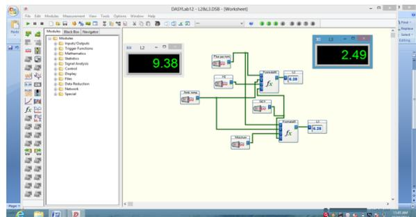
Fig. 4: Application program to monitor L<sub>2</sub> and L<sub>3</sub>
