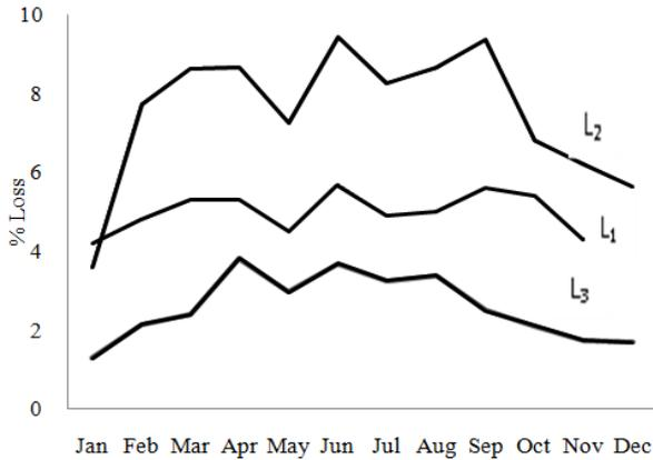
Fig. 1: Month wise percentage boiler losses (L<sub>1</sub>, L<sub>2</sub> and L<sub>3</sub>)
