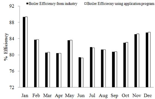
Fig. 9: Month wise comparison of boiler efficiency
