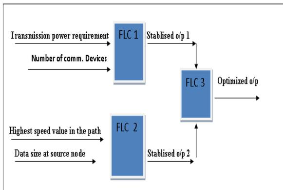
Fig 1 . Inputs to Fuzzy Logic Controller
