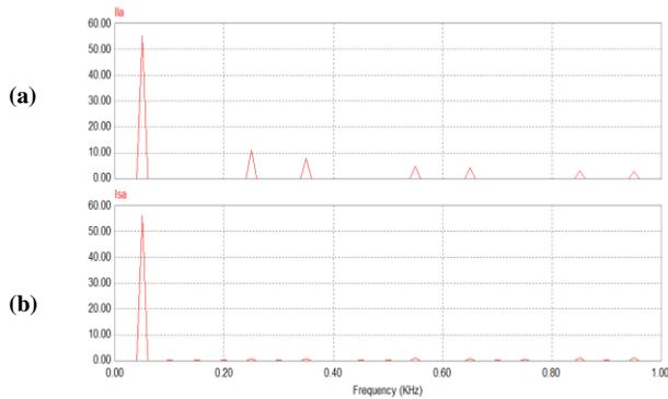
Fig. 10 Harmonic spectrum for Load-1 using GIPT (a) load current of phase-a (b) source current of phase-a
