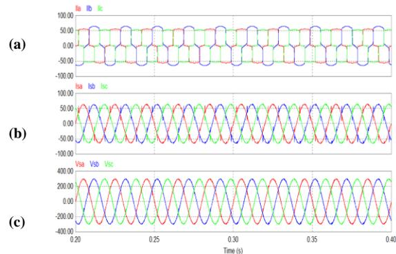
Fig. 8 Simulation waveform for Load-3 using GIPT (a) three phase load current (b) three phase source current (c) three phase source voltage
