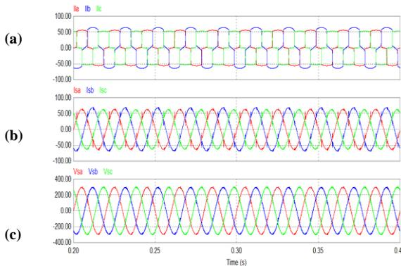
Fig. 5 Simulation waveform for Load-3 using  $p$ - $q$  theory (a) three phase load current (b) three phase source current (c) three phase source voltage
