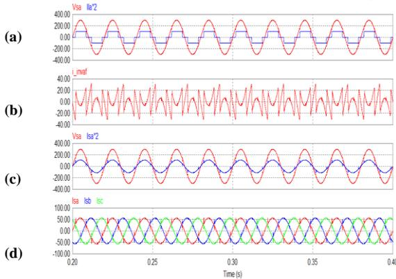
Fig. 3 Simulation waveform for Load-1 using  $p$ - $q$  theory (a) load voltage and load current of phase-a (b) reference current (c) source voltage and source current of phase-a (d) three phase source current
