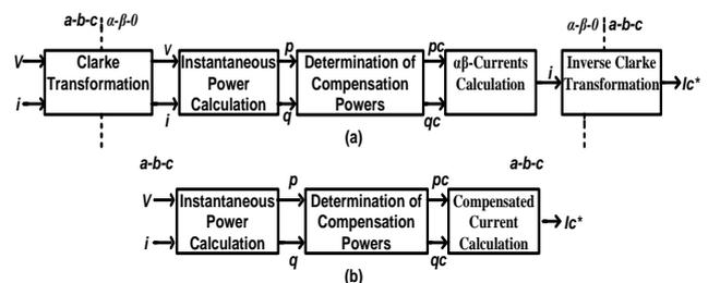
Fig. 2 Control algorithm (a) p-q theory (b) GIPT
