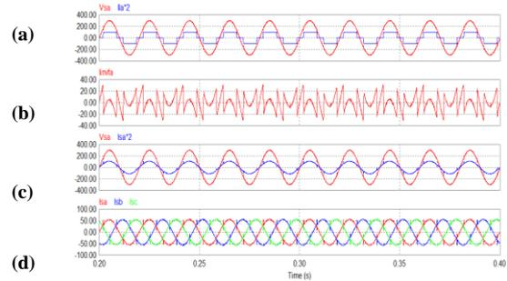
Fig. 6 Simulation waveform for Load-1 using GIPT (a) load voltage and load current of phase-a (b) reference current (c) source voltage and source current of phase-a (d) three phase source current
