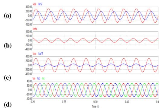
Fig. 7 Simulation waveform for Load-2 using GIPT (a) load voltage and load current of phase-a (b) reference current (c) source voltage and source current of phase-a (d) three phase source current
