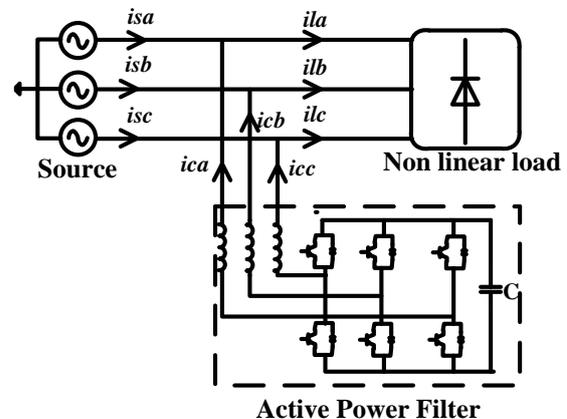
Fig. 1 System diagram of a VSI-SAPF
