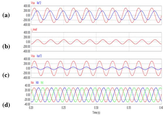
Fig. 4 Simulation waveform for Load-2 using  $p$ - $q$  theory (a) load voltage and load current of phase-a (b) reference current (c) source voltage and source current of phase-a (d) three phase source current
