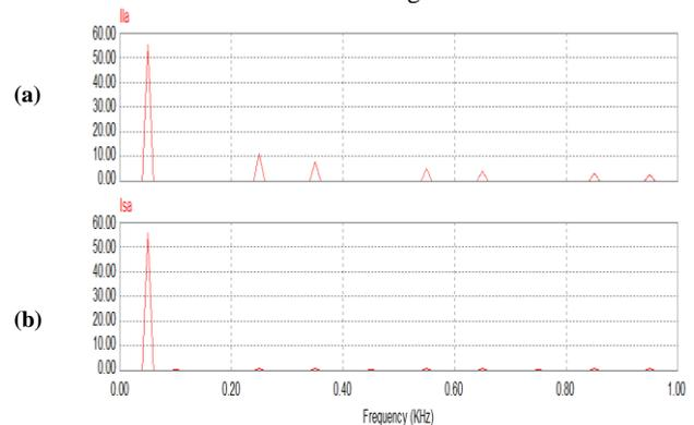
Fig. 9 Harmonic spectrum for Load-1 using  $p$ - $q$  theory (a) load current of phase-a (b) source current of phase-a
