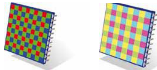
Fig. 4: Bayer array color filter and CMYK color filter array
