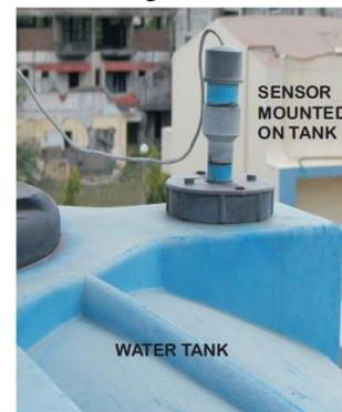
Fig. 4. Mechanical Set-up of the Sensor
