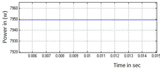
Fig.7. Waveform for maximum power tracked by the MPPT controller
