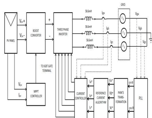
Fig.1. Block diagram of grid connected PV array fed inverter.
