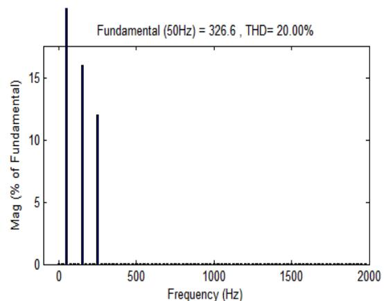
Fig.11. Frequency spectrum of the grid voltage.
