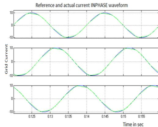
Fig.18. Waveform for reference and actual current synchronization.
