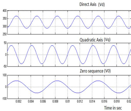
Fig.13. Output waveform of abc-dq0 transformation.
