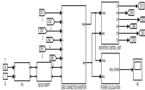
Fig.3. Simulation of grid connected PV array fed inverter.
