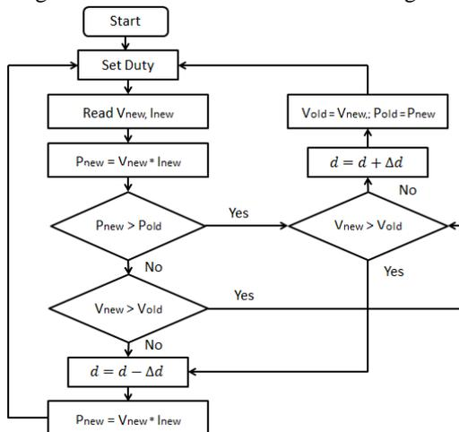
Fig.2. Flowchart for P&O based MPPT algorithm.
