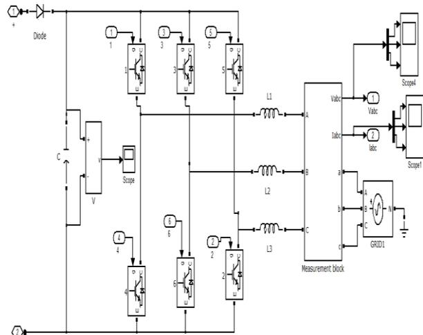
Fig.9. Sub-system for grid tied inverter
