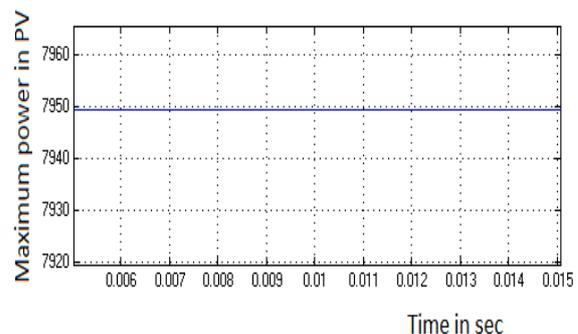
Fig.5. Waveform for maximum power transferred from PV array.
