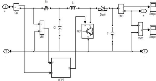
Fig.6. Sub-system for boost converter with MPPT controller.
