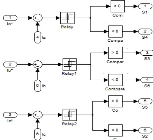
Fig.20. Subsystem of hysteresis current controller.
