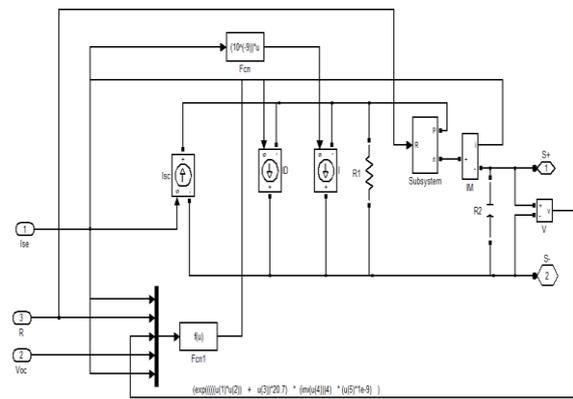
Fig.4. Sub-system for PV array circuit.
