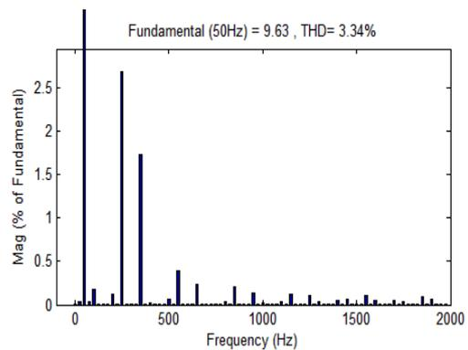
Fig.19. Frequency spectrum of the grid current.
