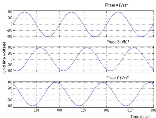
Fig.15. Output waveform of average dq0 to reference voltage.
