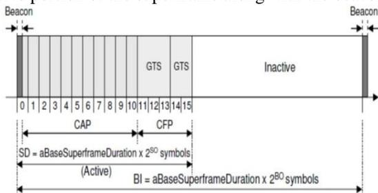
**Fig 4. Superframe structure in IEEE 802.15.4 standard**
