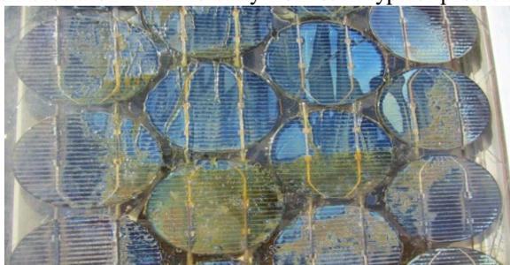
Fig. 7: Degradation of PV module
