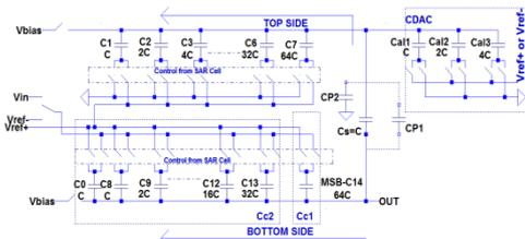
Fig. 7 Unit Split-Capacitor DAC with mismatch calibration
