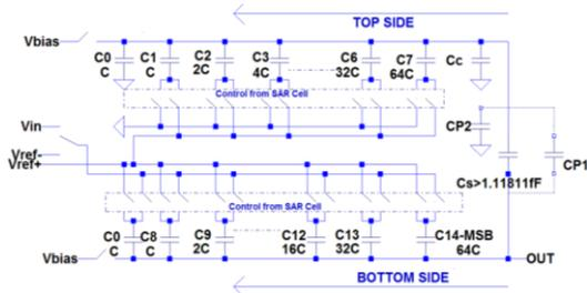
Fig. 5 Split-Capacitor DAC with mismatch calibration
