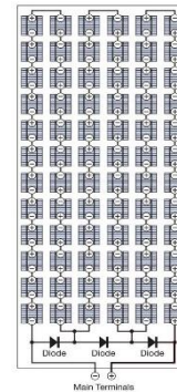
Fig. 10 Bypass diodes in 72 cells module
