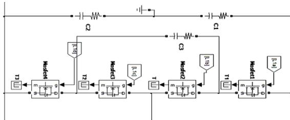
Figure 2: Flying capacitor multi-level inverter limb per phase
