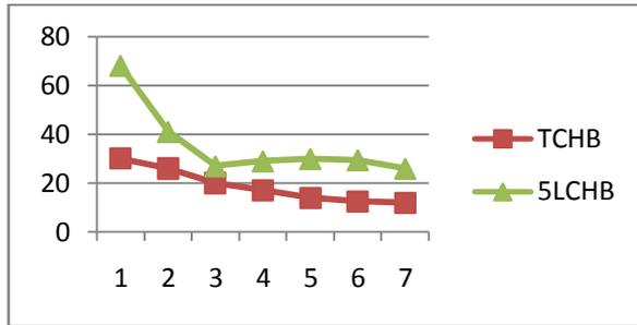
Fig. 9: Line voltage THD of the TCHB inverter and CHB multilevel inverters.
