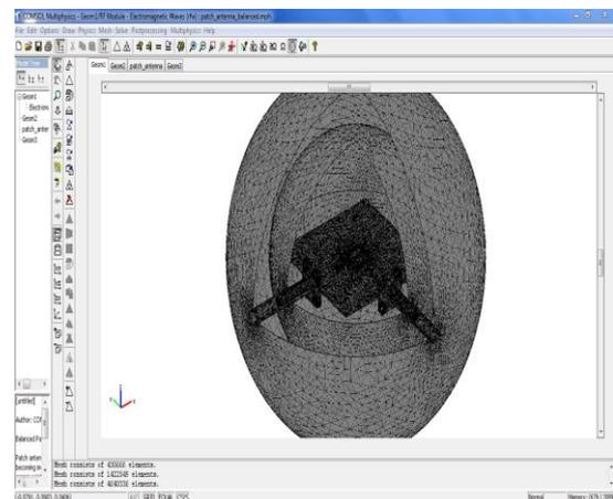
Fig. 5. 3<sup>rd</sup> refinement with 4640336 elements
