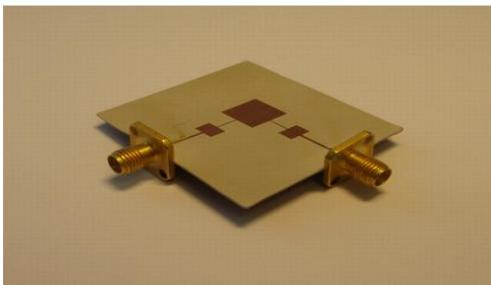
Fig. 2. Fabricated patch antenna [15,16]
