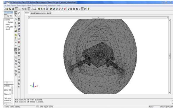
Fig. 3. 1<sup>st</sup> refinement with 430666 elements
