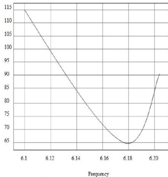
Fig. 10. Antenna Impedance versus frequency
