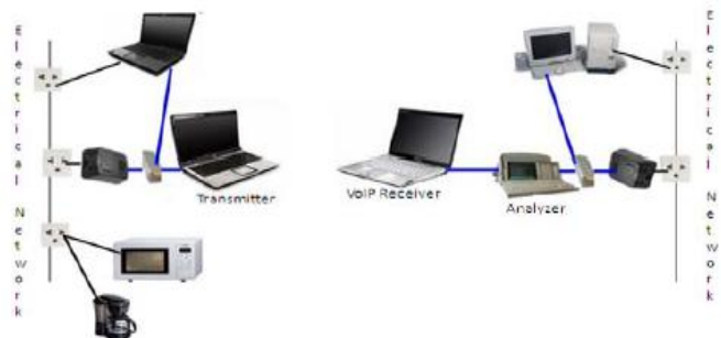
Figure 9.2 - LSCDN USING PLC
