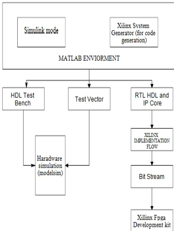
Figure: Block Diagram of System Generator
