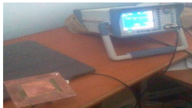
Fig.4 Setup used to evaluate the antenna
