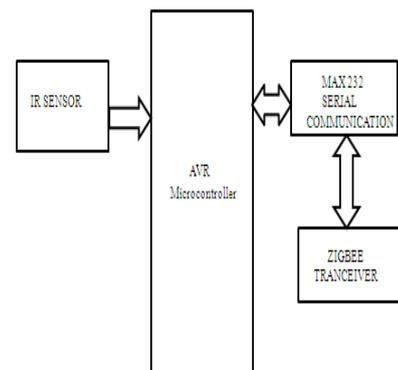
Fig-3. Block diagram of sensor node
