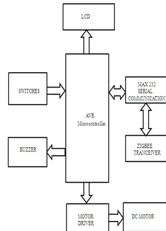
Fig-1 Block diagram of unit at train
