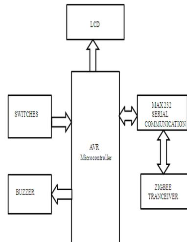
Fig -2. Block diagram of unit at station
