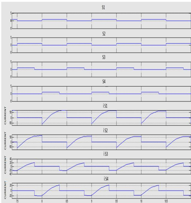
Fig 10 : Current across each switch during switching
