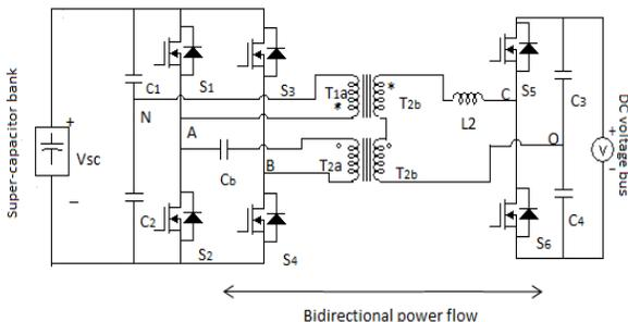
Fig 4: Converter in SC power mode and SC recharge mode
