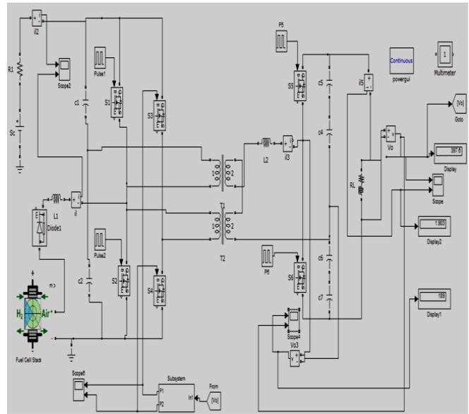
Fig 11: Simulink diagram of the proposed dc-dc converter for constant output voltage
