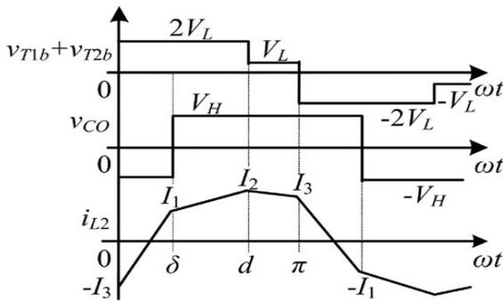
Fig 5: operating waveforms in boost mode when  $0 \leq \delta \leq d$  [11]
