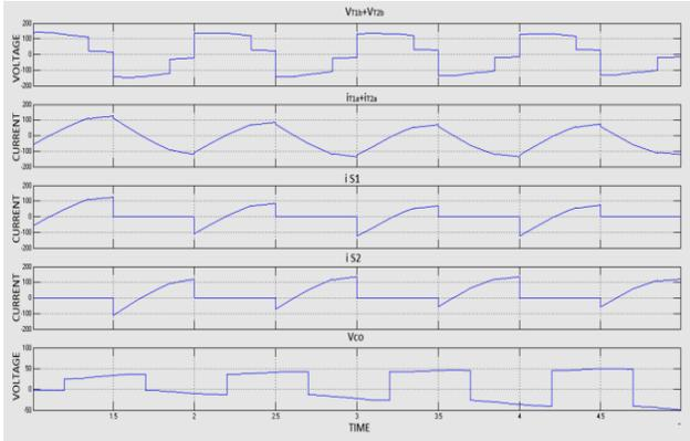
Fig8: Voltage and current waveforms for SC power mode
