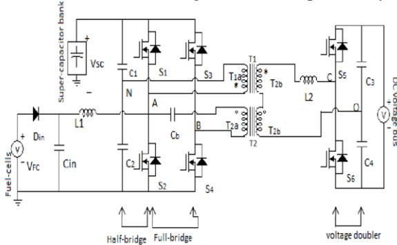
Fig 2: Proposed hybrid bidirectional dc-dc converter topology
