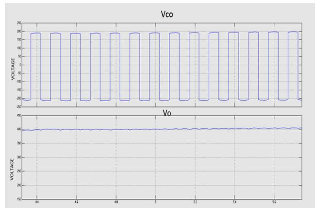
Fig 12: Input & output voltage waveform across voltage doubler circuit
