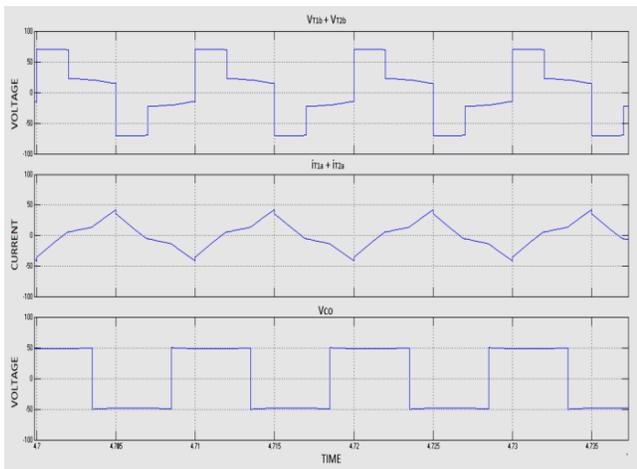
Fig 9: Voltage and current waveforms for SC recharge mode
