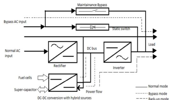
Fig 1: Block diagram of a dual conversion UPS system based on FC & SC
