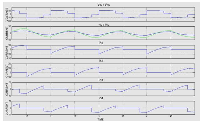
Fig 7: Voltage and current waveforms for boost mode
