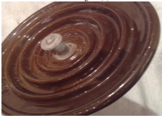
Fig. 2: A photograph of cap and pin type porcelain insulator's creepage distance (C).
