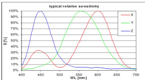
Fig3.5 Spectral characteristic
