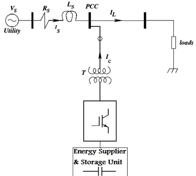
Fig 2 Schematic diagram of FD-STATCOM
