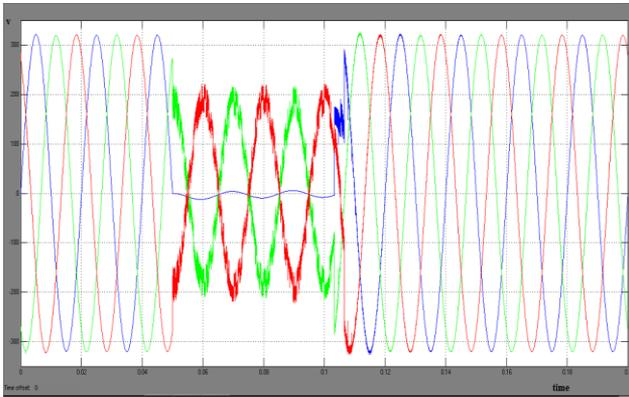
Fig 5 Voltage during DLG fault with out statcom
