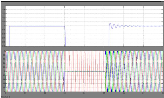
Fig 6 Voltage during SLG fault
