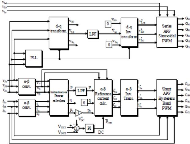
Fig 3 controller blockdiagram
