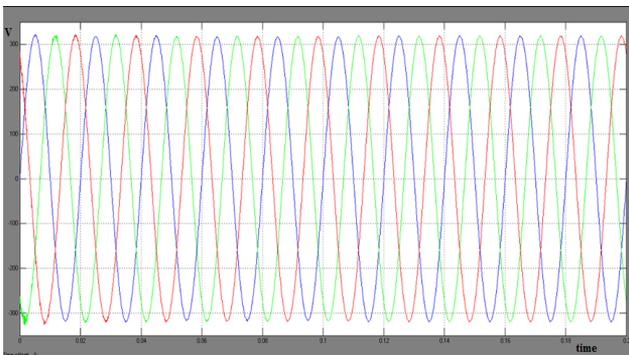
Fig 7 Compensated voltage under Islanding condition
